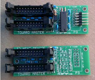
a 65SIB device, but also so I could get as many boards as possible for the minimum price at the board house. The picture at the right shows shrouded headers with ejector hooks. Ejector hooks help unplug the IDC without bending the pins.
