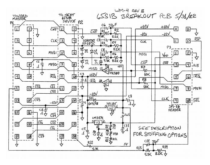
The dots beside each resistor or capacitor indicate the end that's toward the left or top edge of the PCB. Parts and values are shown for interfacing to 3.3V logic on your 65SIB device, translating from the 5V logic of 65SIB.
